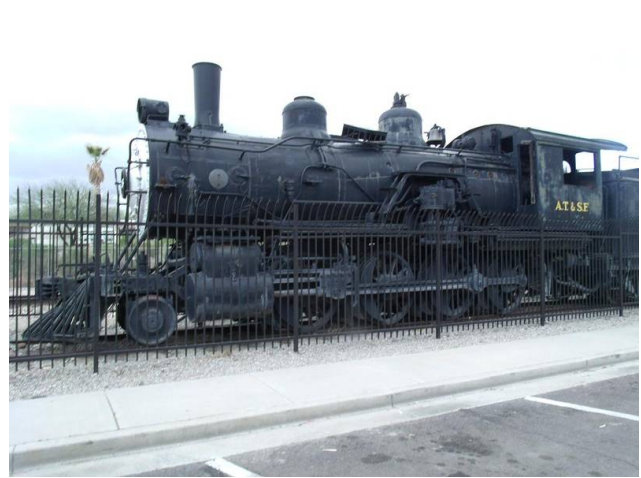
Fig. 48. This locomotive was built around 1890 for the Atchison, Topeka and Santa Fe Railroad. It is a Class 759, 2-8-0. When active, it was used on the main line between Chicago and the west. Engine 761 is located next to the historic Wickenburg train depot (2013-04-09) Tony the Marine (talk); CC BY-SA 3.0 (per Wikimedia Commons) · source
